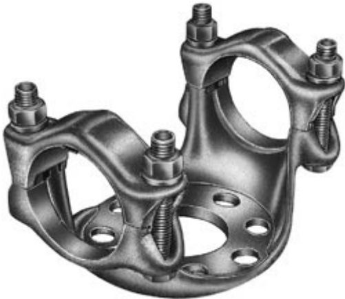
Bus Support, Aluminum Bolted, Slip-Fit or Rigid, 5 IPS/EHIPS ube to Insulator, 5 in B.C.
