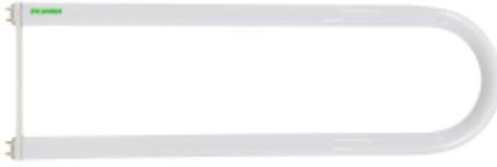
**General Description:** 32W, 22.5" MOL, T8 OCTRON Curvalume fluorescent lamp, 6" leg spacing, 4100K color temperature, rare earth phosphor, 82 CRI, suitable for IS or RS operation, ECOLOGIC
